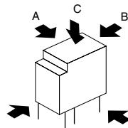
Avoid chucking the center of the relay. In addition, excessive chucking pressure to the pinpoint of the relay should be avoided.
